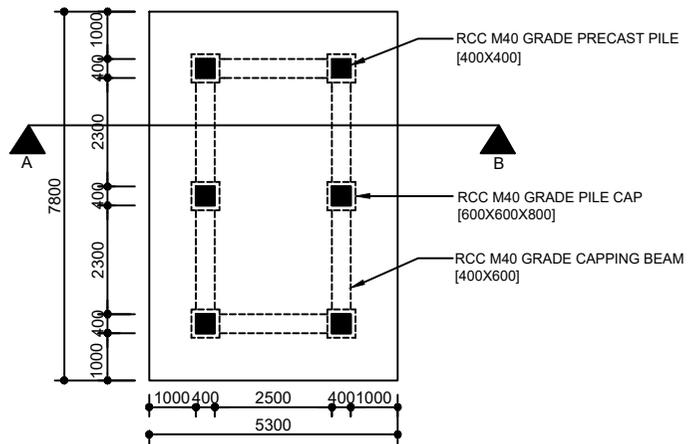
PLAN AT DECK SLAB LEVEL
